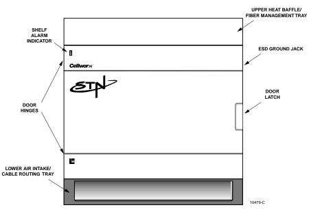
Figure 700-1. Cellworx STN Component Identification
